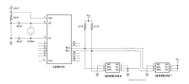
Figure 5 Multi Serial EEPROM( SEEPROM) interfacing
