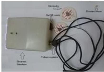
Figure 3. The proposed system components
