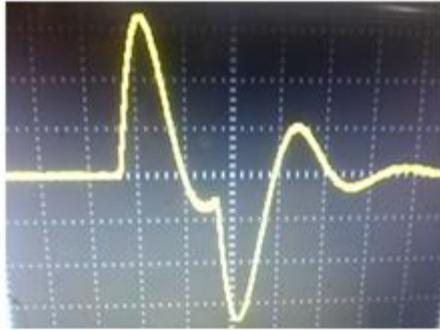
Figure 5. Output waveform of the stimulator.
