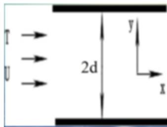
**Figure 1.** Microchannel between two parallel plates
