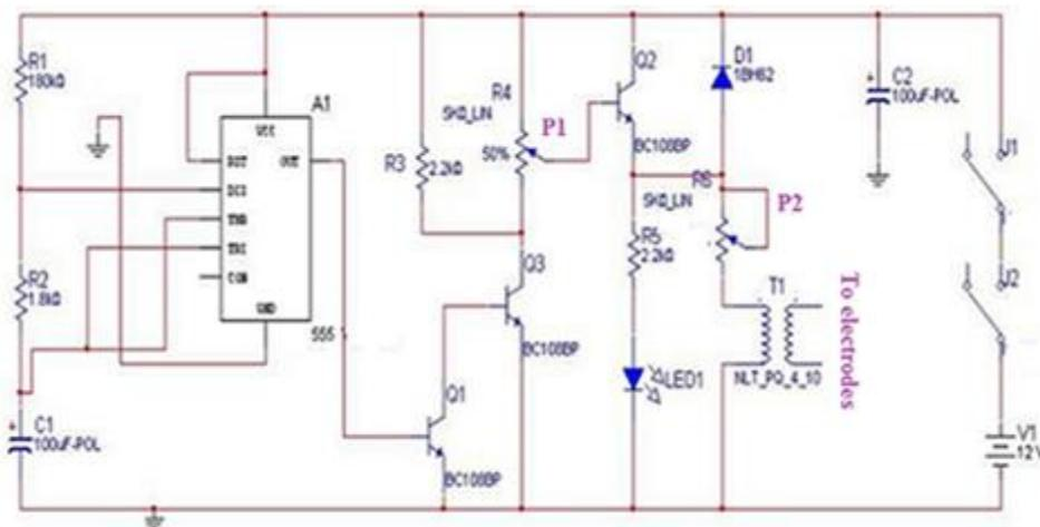
Figure 2. Stimulator proposed electronic circuit.
